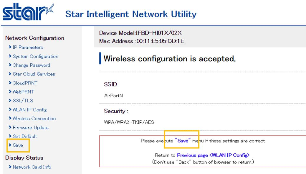
A-8. Select [Save -> Configuration printing -> Restart device] for rebooting with setting print, or [Save -> Restart device] for rebooting without setting print, and click [execute]. Then printer executes reboot and setting is finished.
